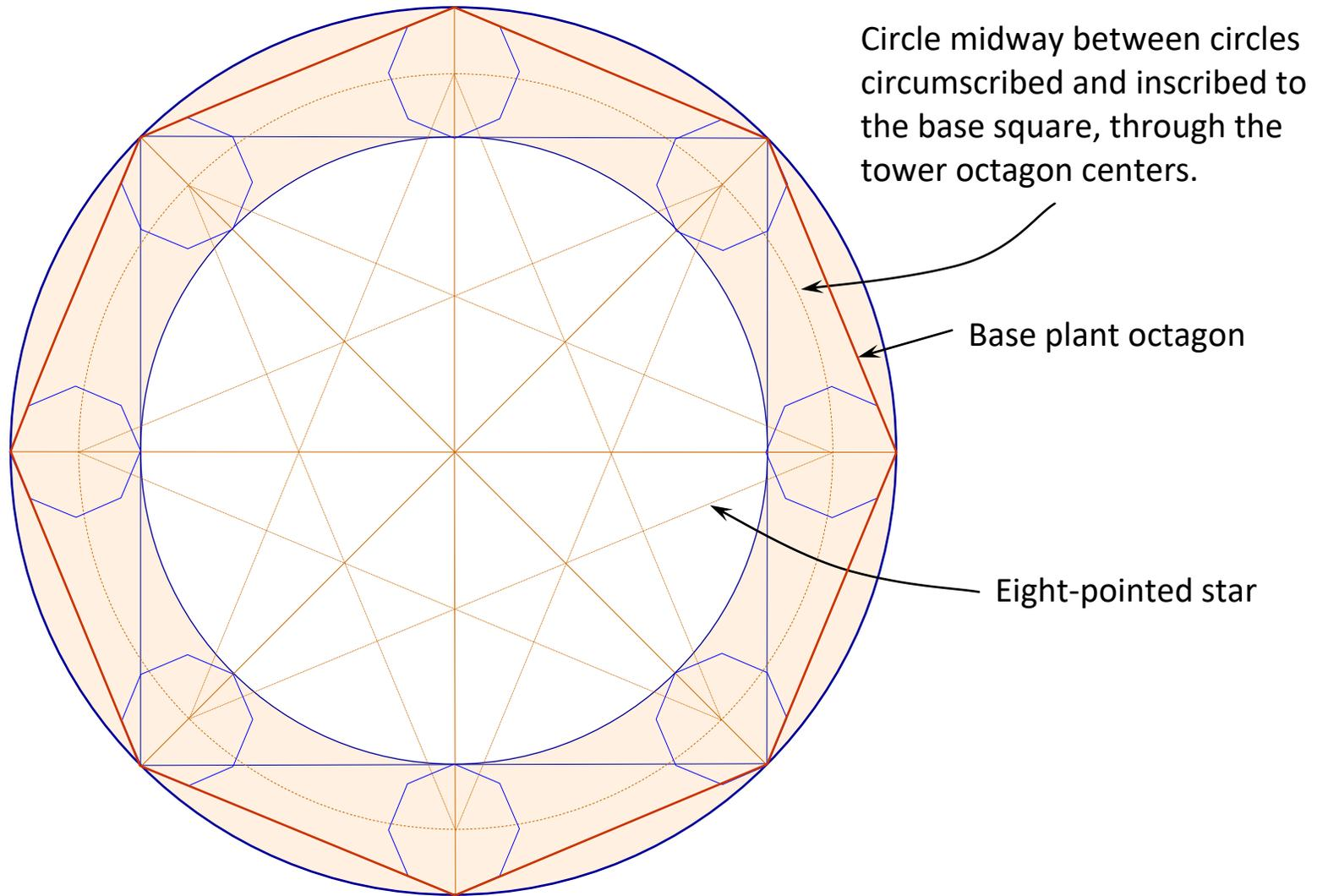
Fig. 6. Base Octagon and Towers in the Tower Space
