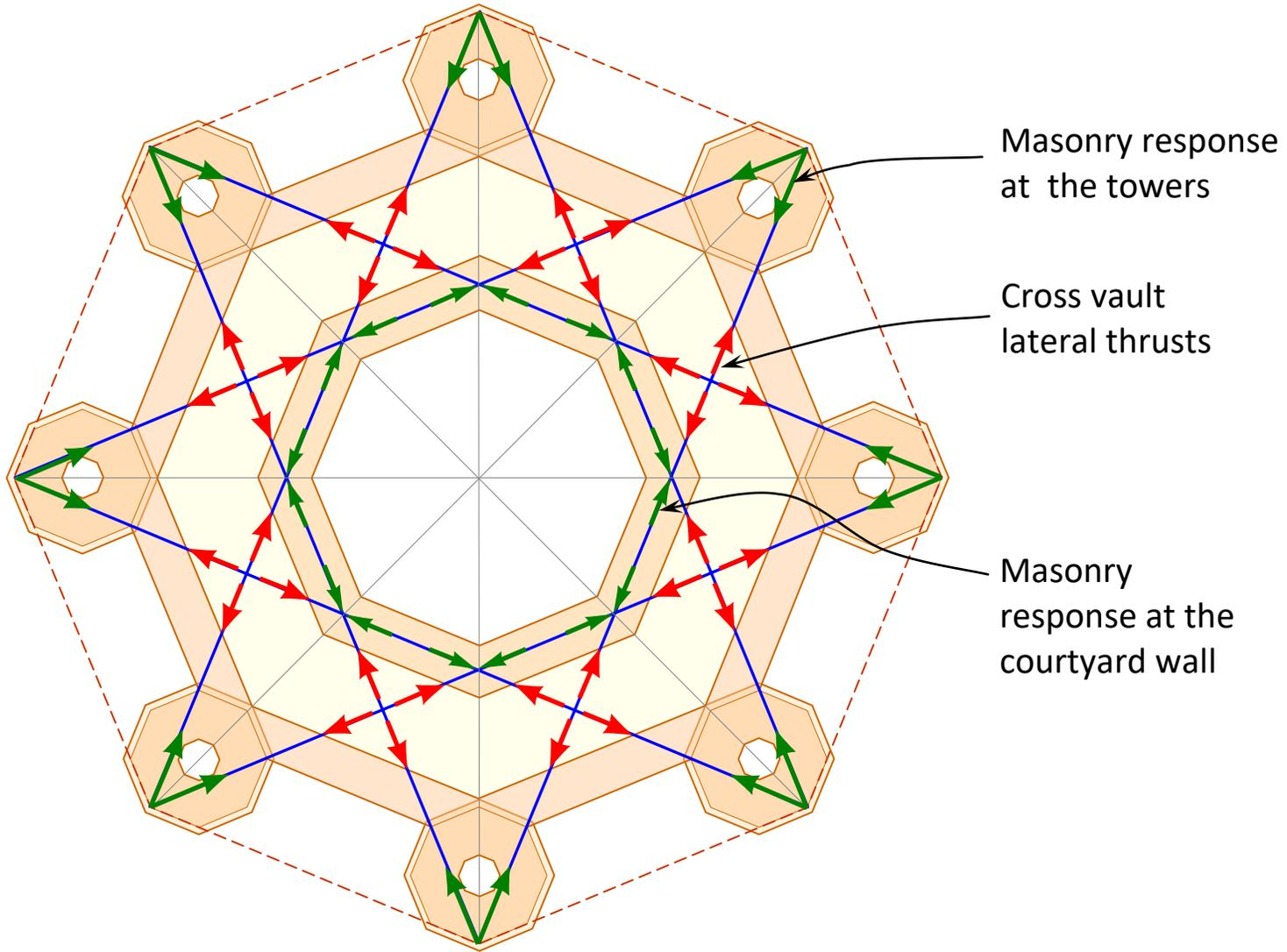
Fig. 7. Cross Vault Lateral Thrust Solution at Castel del Monte
